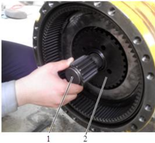
Fig. 3-138 1 Sun gear shaft, 1 piece 2 Friction plate bracket, 1 piece
