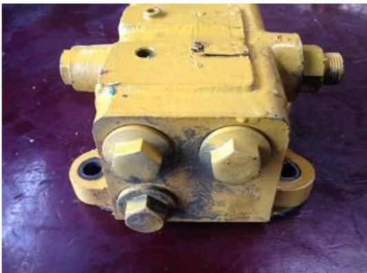
2. Tighten the plug screw of all valve cores.
