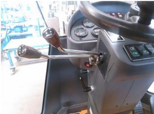
Fig. 2-3 Gear selector
