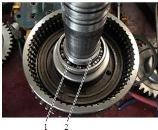
4. Successively install the bearing and the retainer ring onto the clutch shaft.
