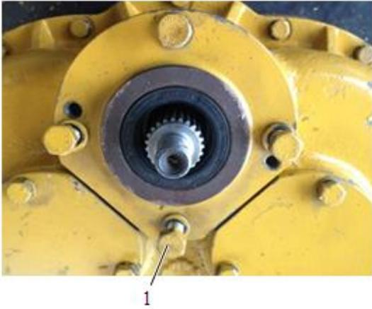
10. Tighten the fixing bolts of input bearing pedestal.
