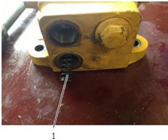
7. Take out the shut-off valve spring and the valve core.
