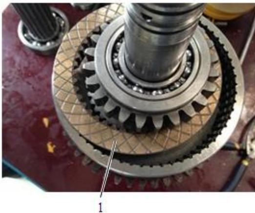
7. Alternatively place internal and outer friction linings into the clutch.
