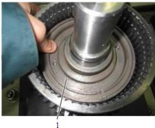
2. Put the piston into the clutch.
