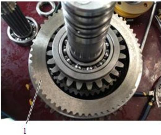
6. Place the outer friction lining into the clutch.
