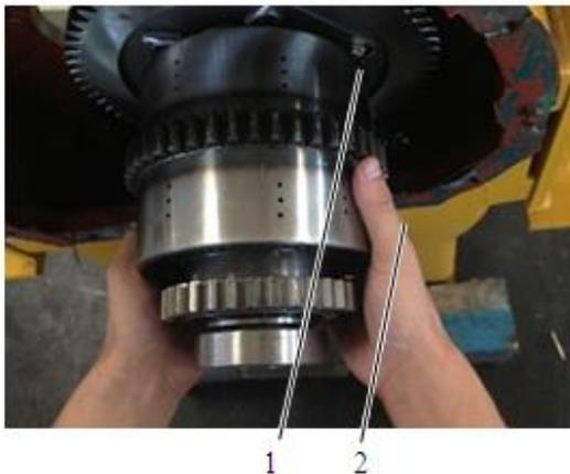
1. With the face connecting the housing with the torque converter upwards, install the high-speed reverse clutch assembly into the housing.
