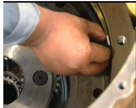
22. Warped the stop pin of isolate plate with screwdriver.
