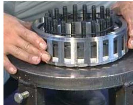
8. Take out the shield ring with circlip pliers.
