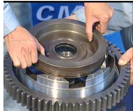
9. Take down the seal ring and rotary oil seal on the direct gear piston by hand.
