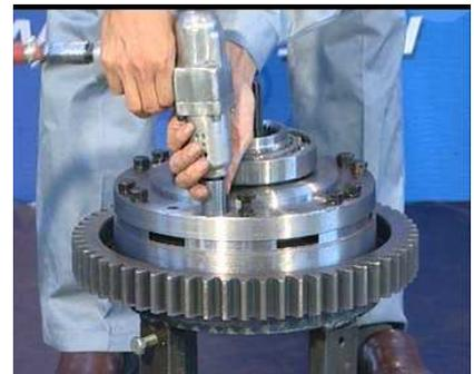
3. Disassemble the connecting bolt.
