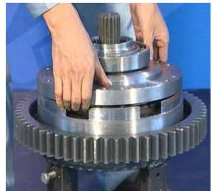
5. Take down the direct gear and three friction plates together.
