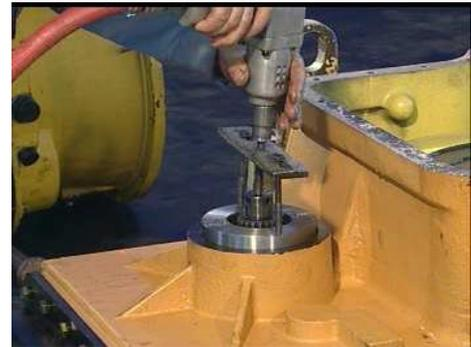
13. Take down the shield ring by axis-shield ring pliers.
