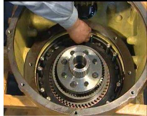
19. Take out the first gear ring and separate the friction plate on it.
