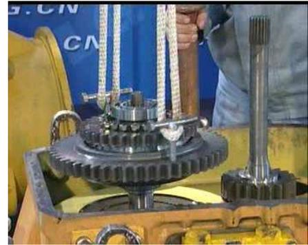
4. Disassemble the third-axis assembly from box body.
