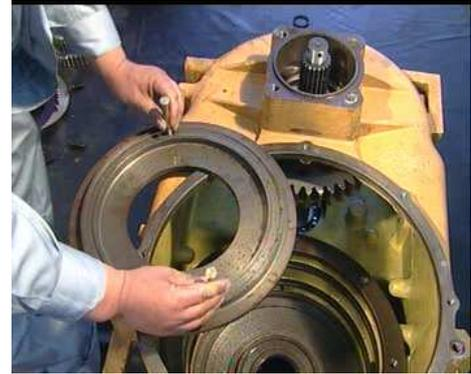
27. Detach the spring seal ring on the box four-axis with circlip pliers.
