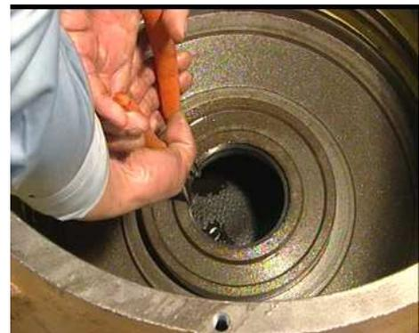
28. Loose the connection screws that fixed the shift pump.
