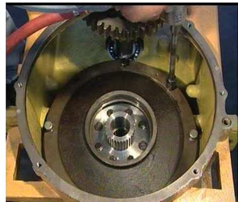
17. Disassemble First gear oil cylinder by hand. Take out the piston, the internal and external seal ring.
