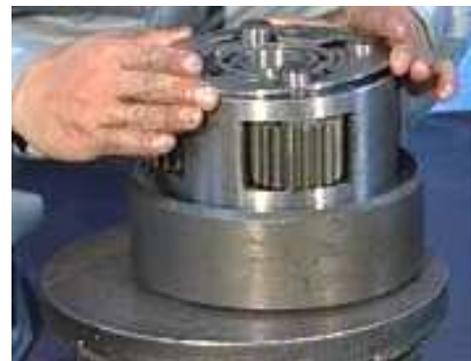
5. Take out the shield ring in reverse ring gear with screwdriver.
