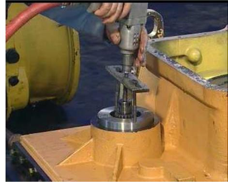
8. Take down the shield ring by axis-shield ring pliers.
