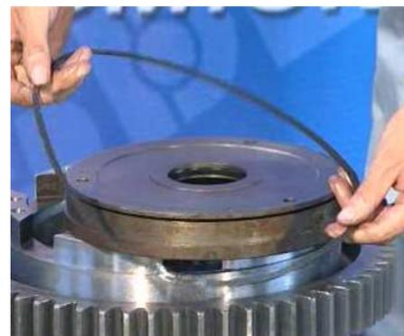
10. Take down the intermediate output gear by hand, separate the direct gear cylinder from the intermediate output gear, then take down the intermediate output gear.
