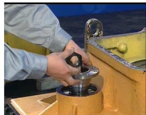
7. Disassemble the oil seal assembly with professional tools.
