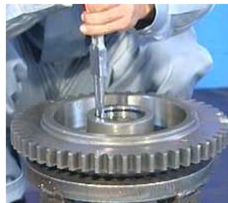
9. Beat the bearing in outer loop gear out with copper rod lightly.
