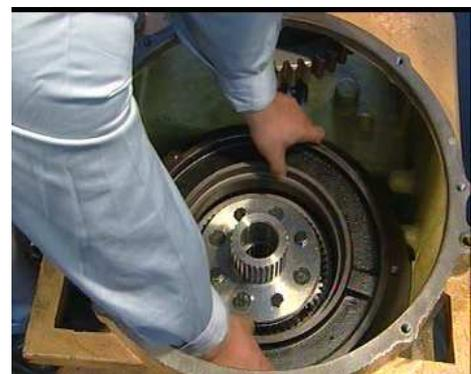
18. Take out the return spring and spring guide pin by hand.
