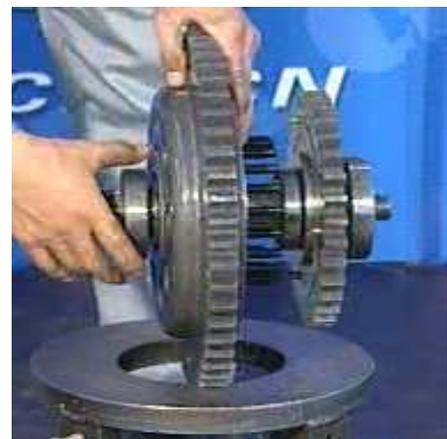
5. Bind the bolts with rubber band, and then take out the isolating ring, inner loop cam and 24 balls and bolts simultaneously.
