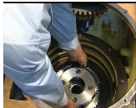
26. Take out the reverse gear piston, internal and external seal ring.
