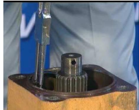
14. Loose the end cover bolts with corresponding specification tools and push end cover away from box with two pusher screws. Top screw: M10.
