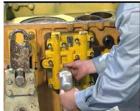
6. Loose the bolts by corresponding specification tools. Take down the stop-pushing gasket and back export flange.
