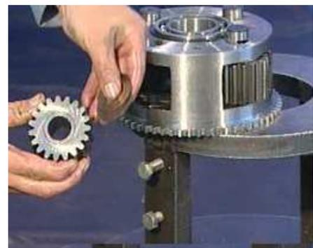
9. Take out the shield ring and needle roller in the planet gear.
