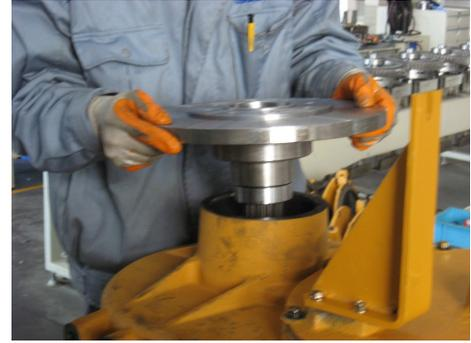
12. Disassemble the oil seal assembly with professional tools.
