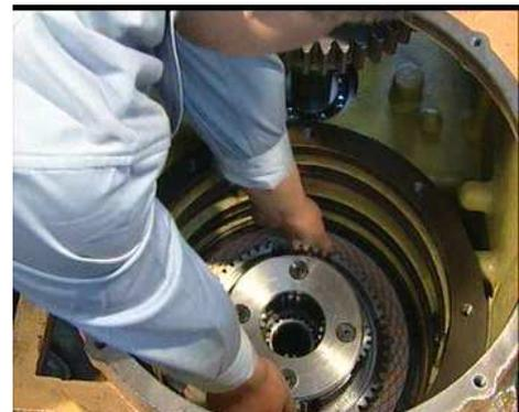
25. Take out the reverse gear planetary carrier assembly by hand.
