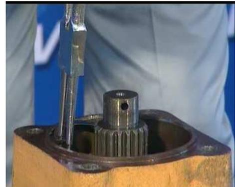
9. Turn the big end surface of transmission box to downward and put the transmission assembly fixed on the carrier.
