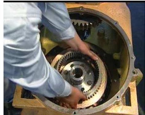
20. Take out the first gear planetary carrier assembly.
