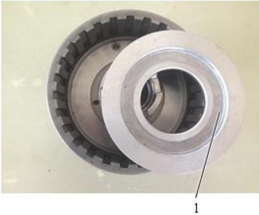
15. Install K4 clutch piston into the clutch.
