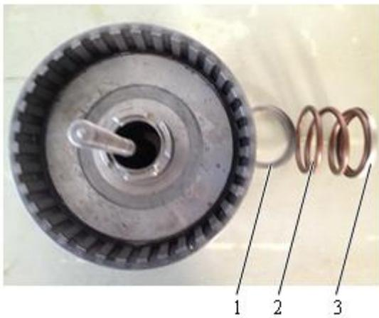
16. Install guide ring and pressure spring into the clutch cylinder.
