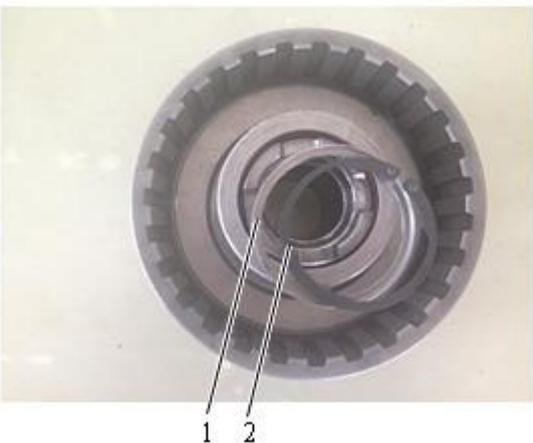
17. Install guide ring and retainer ring.
