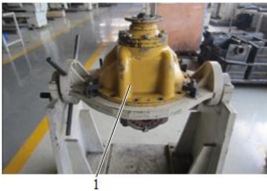
1 Put and fix the main drive on the jig horizontally (with the input flange upward).
