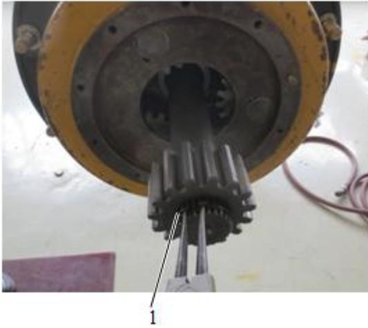
14 Installing the retainer ring
