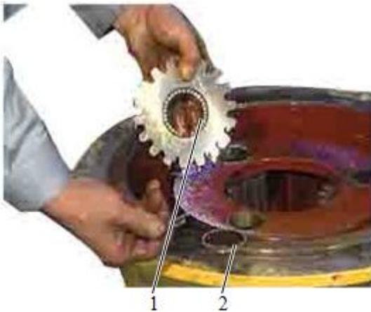
5 Remove the retainer ring and then the needle on the inside wall of the planetary gear.
