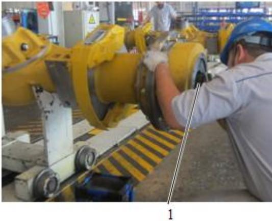
15 Installing the half axle
