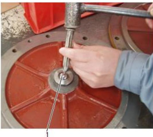
16 Installing the steel ball
