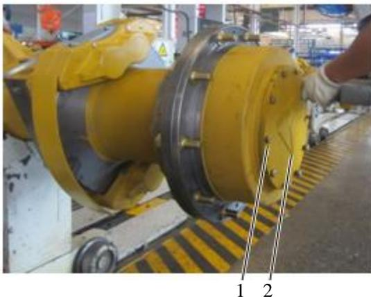
19 Tightening the end cover with bolts and washers
