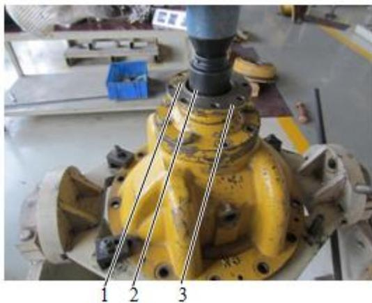
2 Remove the locking nut with appropriate tools, and remove the input flange and the gasket.
