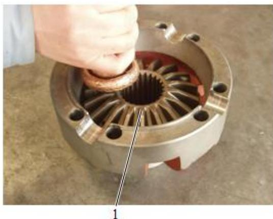
8 Installing face gear
