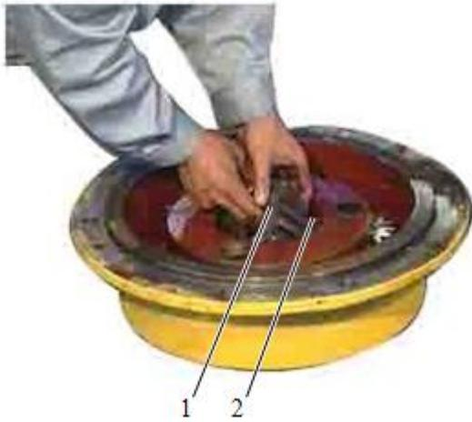
4 Remove the planetary gear and the gasket.
