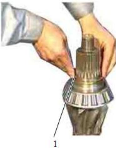
5 Remove the adjusting gasket.
