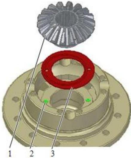
9 Installing the face gear
