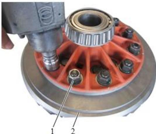
2 Loosen the nut connecting the driven spiral bevel gear and the right differential housing, and remove the driven spiral bevel gear.
