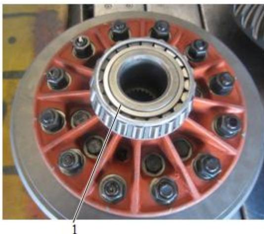
3 Remove the bearings on the left and the right differential housings.
