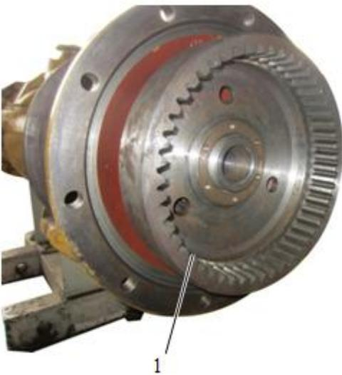
16 Removing the inner ring gear
