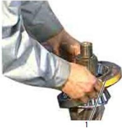
3 Remove the bearing sleeve.
