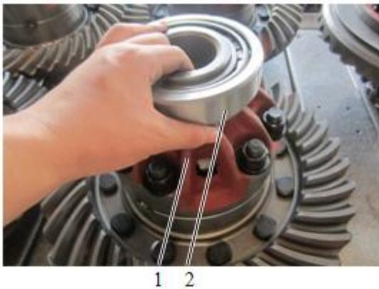
14 Install a roller bearing at the outer bearing position of the left differential housing.
