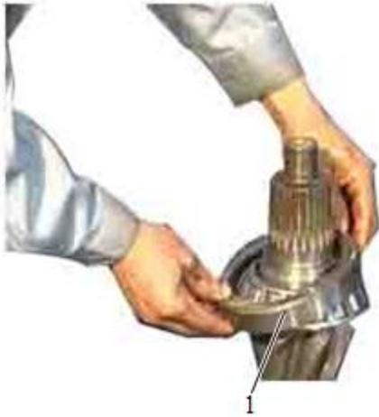
4 Remove the bearing outer ring.
