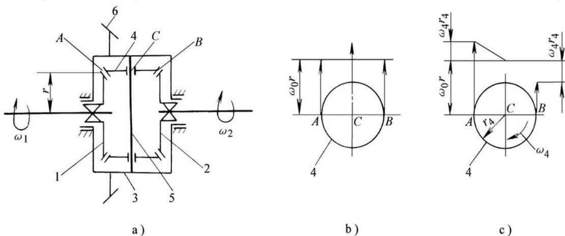
Fig. 2-4 Differential Principle
