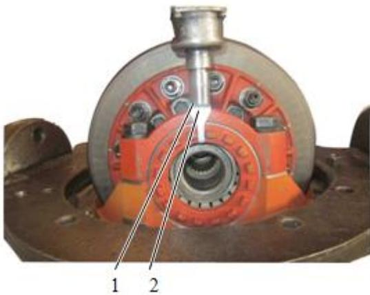
8 Remove the bolt and the washer fixing the locking plate, and remove the locking plate.
