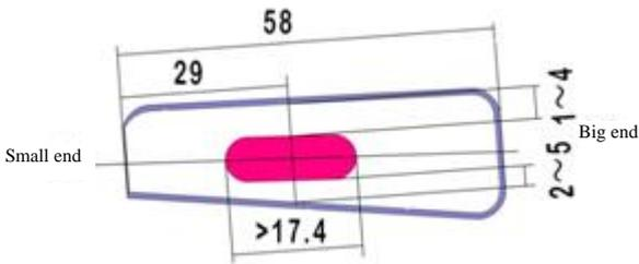
Concavity of Spiral Bevel Gear
