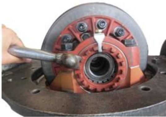
7 Make a mark in order to fit it into the original position when reassembling.
